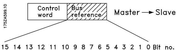
The frequency reference value is transmitted to the frequency converter in the form of a 16-bit word. The value is transmitted as a whole number (0-32767). 16384 (4000 Hex) corresponds to 100%. (Negative figures are formed by means of 2's complement.)
