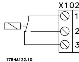
See parameter 323 (relay output) for programming of relay output.
