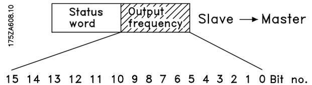
The value of the actual output frequency of the frequency converter is transmitted in the form of a 16- bit word. The value is transmitted as a whole number (0-32767). 16384 (4000 Hex) corresponds to 100%. (Negative figures are formed by means of 2's complement).
