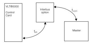
Communication time ( $t_{com}$ ) depends on the type of master in use, the total number of bytes transmitet to all slaves and the total length of the INTERBUS Cable.
