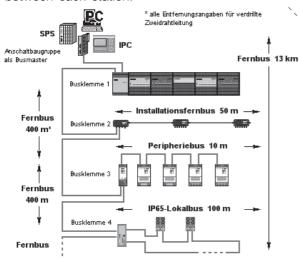
The locale bus system enables the user to establish communication to Input/output devices throught a single twisted pair of Cables. This type of comunication is typical used the simple devices E.g. Digital I/O devices.
