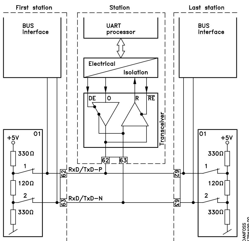
It is important to terminate the bus line correctly. Mismatches of the impedance may lead to reflections in the line and cause incorrect transmissions.
