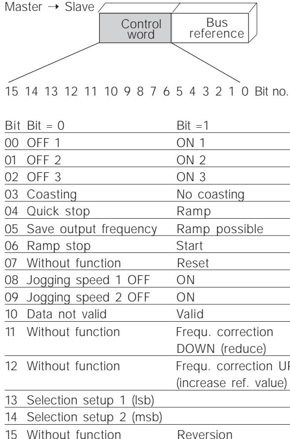
If "Profidrive" has been selected, then a two-part start command has to be observed when the start is released (turn-on lock-out: bit 0).
