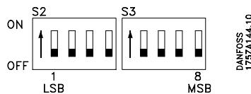
The setting of an address through parameter 918 is only possible when the address switches are set to 0 or > 126.
