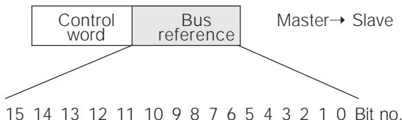
The frequency reference value is transmitted to the frequency converter in the form of a 16-bit word. The value is transmitted in integers (0-32767). 16384 (4000 Hex) corresponds to 100%. (Negative numbers are formed with the aid of the two's complement.)
