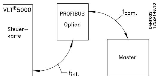
The communication period ( $t_{com.}$ ) depends on the respective transmission speed (baud rate) and the type of master being used. The shortest achievable communication period is approximately 30  $\mu$ sec per slave with the VLT PROFIBUS option when DP communication with a data quantity of 4 bytes (PPO type 3) at 12 Mbaud is used. The communication period increases with more data or lower transmission speeds.
