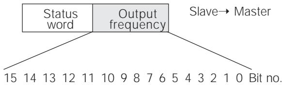
The value of the current output frequency of the frequency converter is transmitted in the form of a 16-bit word. The value is transmitted in integers (0-32767). 16384 (4000 Hex) corresponds to 100%. (Negative numbers are formed with the aid of the two's complement.)
