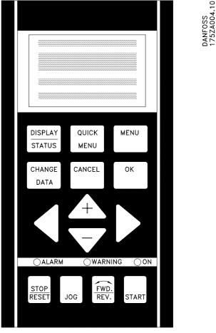
1st line shows up to 3 measurements continuously in normal operating status or a text which explains the 2nd line.
