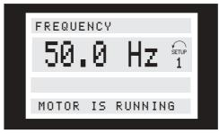
Line 2 gives the data value of an operating variable with related unit, and line 1 provides a text which explains line 2, cf. table. In the example, Frequency has been selected as variable via parameter 009. During normal operation another variable can immediately be read out by using the [+/-] keys.
