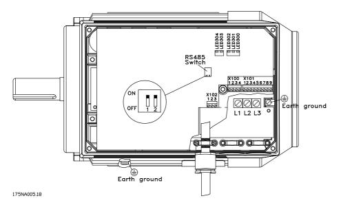
Terminal arrangement (for installation see quick setup, MG.03.AX.62)
