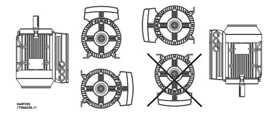
FC motors must be installed with adequate access for routine maintenance. A minimum of 0.75m of working space around the motor is recommended. Adequate space around the motor, particularly at the fan inlet (50 mm), is also necessary to facilitate airflow. Where several FC motors are installed in close proximity, care must be taken to ensure that there is no recirculation of exhausted warm air. Foundations must be solid, rigid and level.
