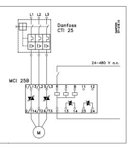
The thermostat is connected in series with the control circuit of the main contactor When the temp. of the heat sink exceeds 100°C the main contactor will be switched OFF. This circuit requires manual reset to restart the motor.
